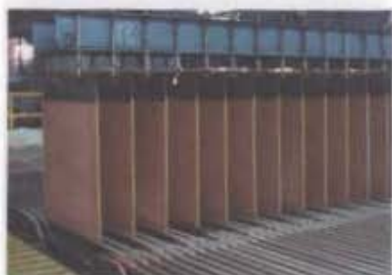
Pure copper plates produced by electrolysis
